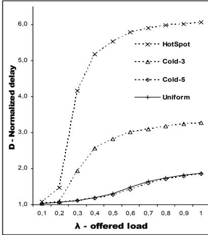
Figure 5. Normalized delay of a single-priority, double-buffered, 6-stage MIN under hotspot traffic
