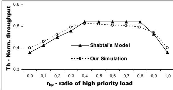
Figure 2. Total normalized throughput of a dual-priority, single-buffered, 6-stage MIN
