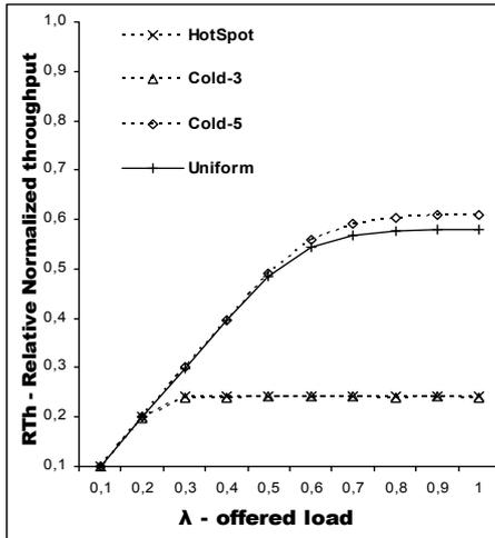
Figure 3. Normalized throughput of a single priority, double-buffered, 6-stage MIN under hotspot traffic
