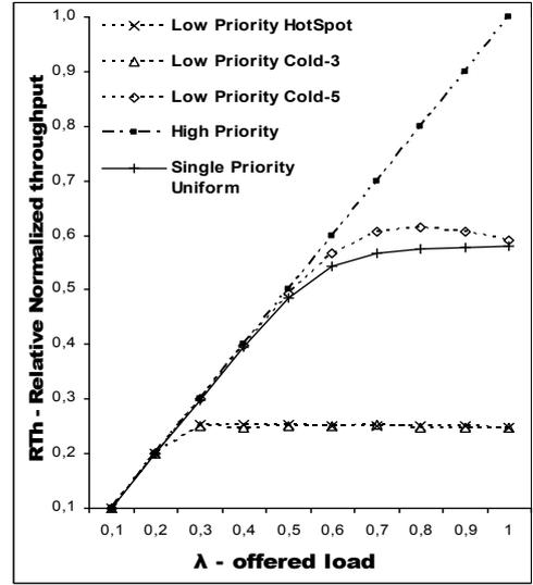
Figure 4. Normalized throughput of a dual-priority, double-buffered, 6-stage MIN under hotspot traffic
