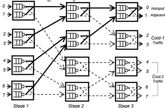
Figure 1. An  $8 \times 8$  delta-2 network with hotspot traffic
