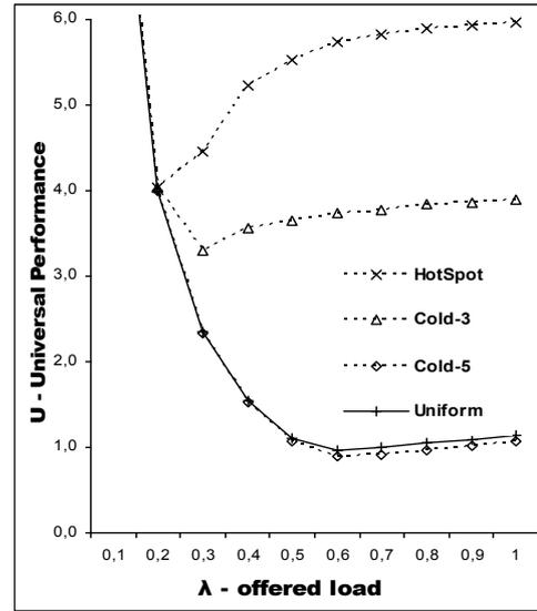
Figure 7. Universal performance of a single-priority, double-buffered, 6-stage MIN under hotspot traffic
