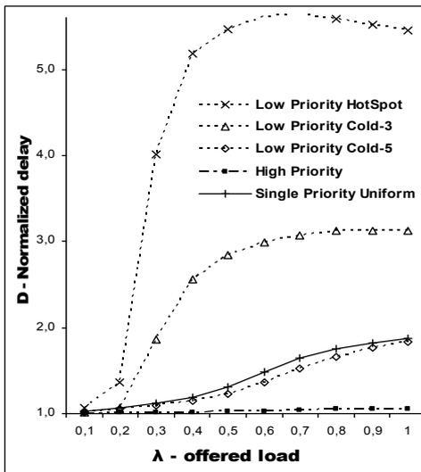
Figure 6. Normalized delay of a dual-priority, double-buffered, 6-stage MIN under hotspot traffic
