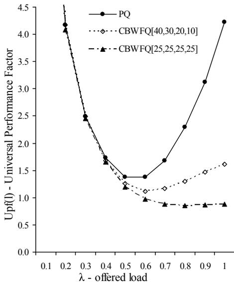
Figure 17. Universal performance factor for low-priority packets vs. offered load
