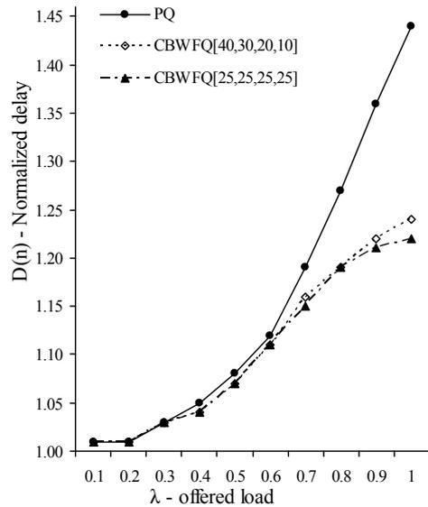
Figure 12. Normalized delay for normal-priority packets vs. offered load
