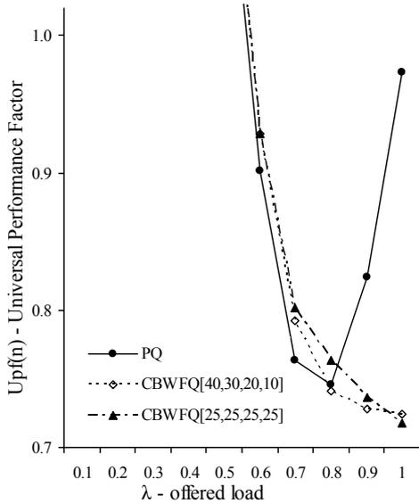
Figure 16. Universal performance factor for normal-priority packets vs. offered load
