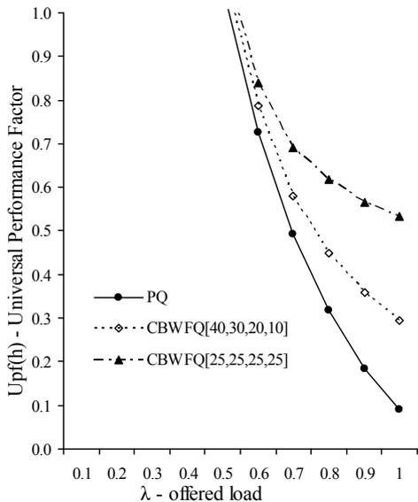
Figure 14. Universal performance factor for high-priority packets vs. offered load
