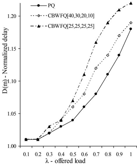
Figure 11. Normalized delay for medium-priority packets vs. offered load
