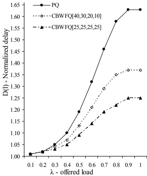
Figure 13. Normalized delay for low-priority packets vs. offered load
