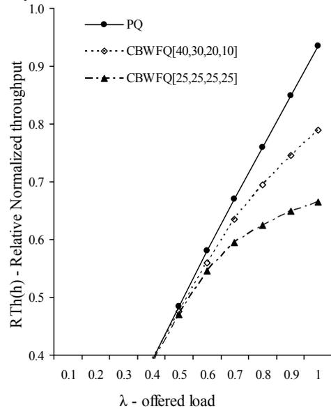
Figure 6. Relative normalized throughput for high-priority packets vs. offered load
