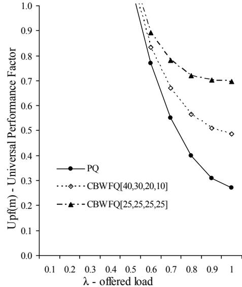
Figure 15. Universal performance factor for medium-priority packets vs. offered load
