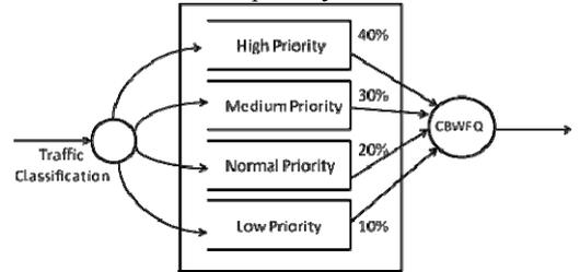
Figure 2. Class-based weighted fair queuing algorithm
