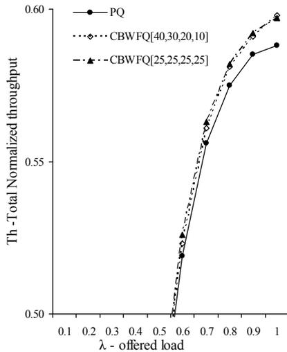
Figure 5. Overall MIN throughput under varying scheduling algorithms and queue weight settings
