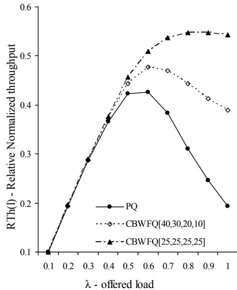
Figure 9. Relative normalized throughput for low-priority packets vs. offered load
