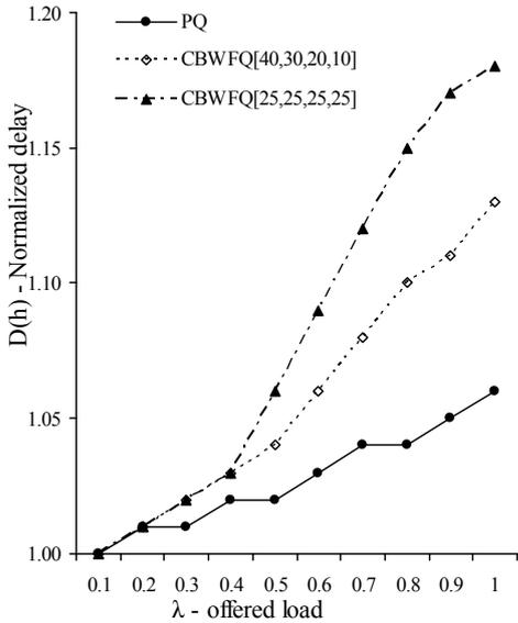
Figure 10. Normalized delay for high-priority packets vs. offered load
