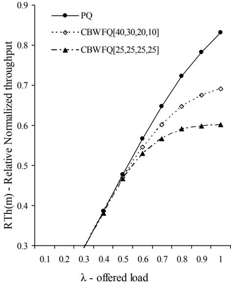
Figure 7. Relative normalized throughput for medium-priority packets vs. offered load
