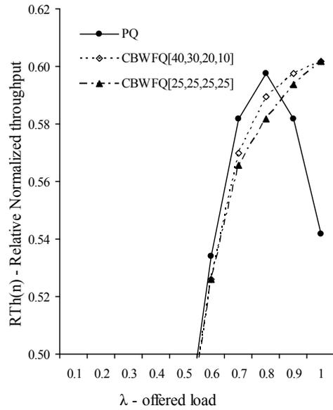
Figure 8. Relative normalized throughput for normal-priority packets vs. offered load
